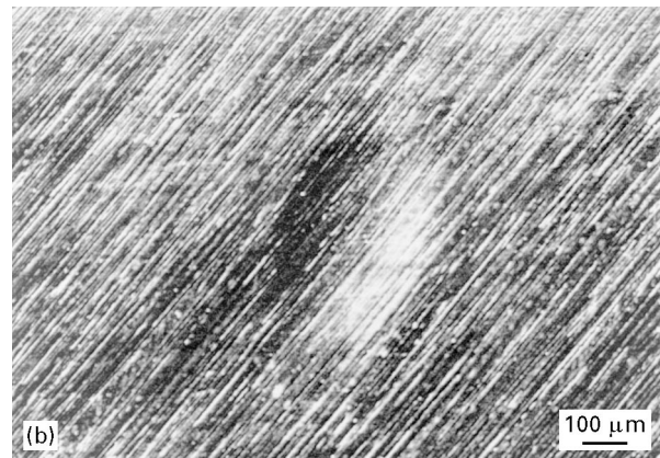
Figure 13 The residual indented area by scanning electron microscopy for (a) the N fibre orientation ( F = 100 ) and (b) the P fibre orientation ( F = 40 ).
